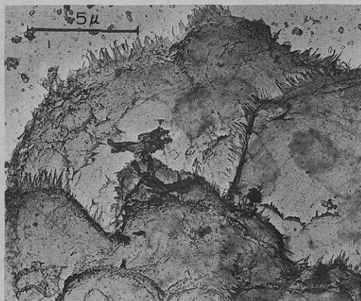
Figure 1. Polypropylene fibrils growing on the lateral edges and on surface defects of the \alpha -TiCl 3 crystal. Carbon replica. Electron micrograph.
